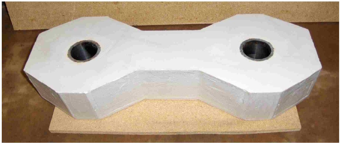
Figure 2 Hydro-Stone TB Specimen Dog Bone 1
