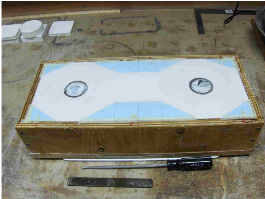
Figure 4 Dog Bone 1 after Hydro-Stone TB Pour
