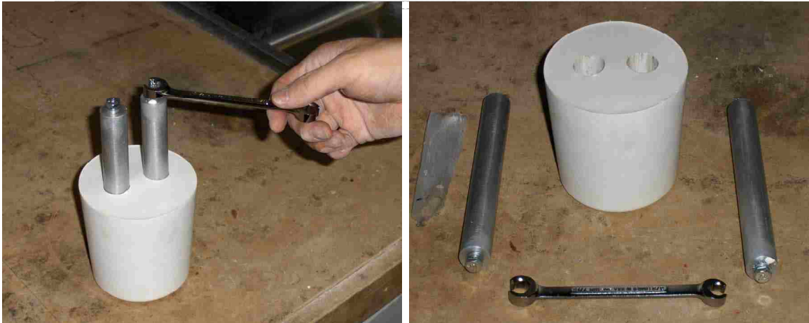
Figure 16 Aluminum Rod Removal Test
