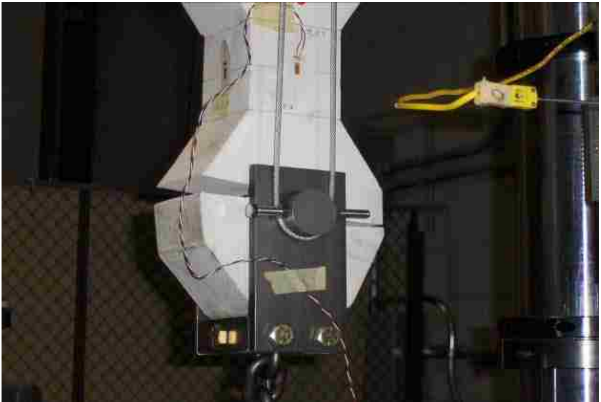
Figure 9 Dog Bone 2 in MTS Testing Machine after Failure
