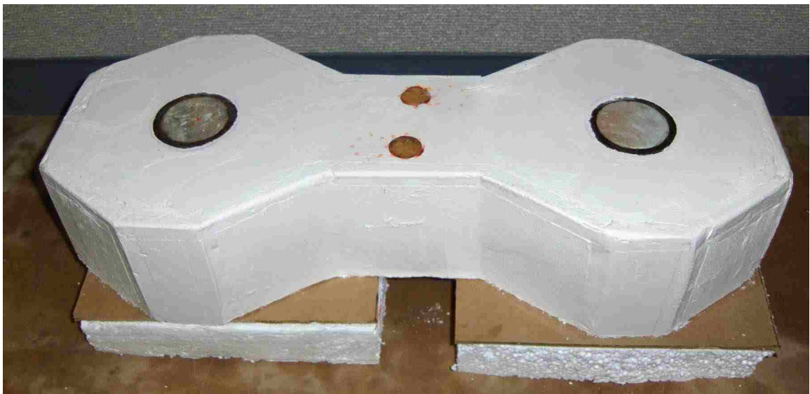
Figure 14 Dog Bone 4 after Mold Removal
