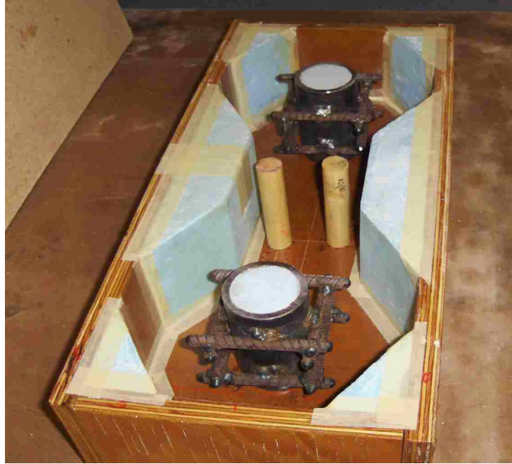
Figure 13 Mold for Dog Bone 4 with Pipes, Bars and Porosity Dowels
