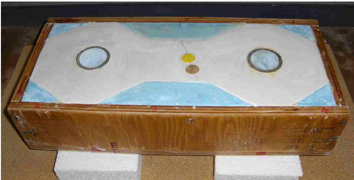
Figure 11 Crack in Dog Bone 3
